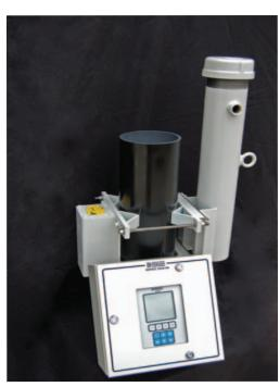
In many applications Ronan's unique RLL technology may be used, significantly reducing the size and cost of the excitation (source). No contact is made to the material, allowing extremely caustic, abrasive or high temperature materials to be safely measured. The density metering system may be installed or removed without disturbing the existing piping and no diverting of the material is required.
