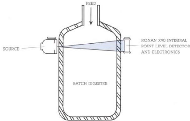
A radiation source is placed opposite a single point detector at a desired level. When the mass of wood chips interrupts the radiation beam, the detector switches state, signaling the operator or a control device. This automatic level indicator assists the operator in reducing cook time and controls the digester product.
